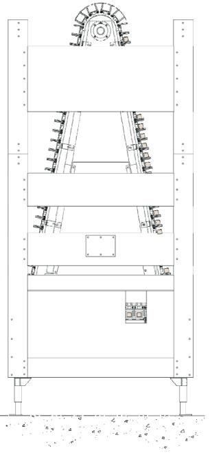
Dillin's "Flex Sweep" Accumulator is a specialized solution for products that would normally be difficult to accumulate through standard means. It's multiple lane infeed accommodates high upstream rates and features open access from the operator side and visibility of accumulated product from all sides.
